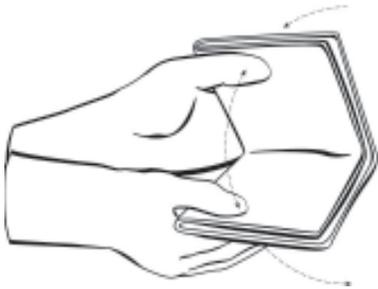
**Step 1:** Quarter-fold Wiper *after* wetting with DI Water. For use with IPA, quarter-fold *prior* to wetting.
